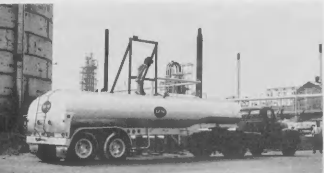
THE FIRST delivery of penetration asphalt for the Princess Beatrix Airport construction project was made Sept. 9. A 9000-barrel tank and special swivel delivery arrangement were constructed south of the Central Tool Room. E PROMER entrega di asphalt pa aeropuerto tumando Beatrix, caminda un proyecto di construcion ta pasando lugar, a worde haci 9 di September. Un tanki di 9000 barril cu su tubo especial ta equipo cu a worde trabá.
